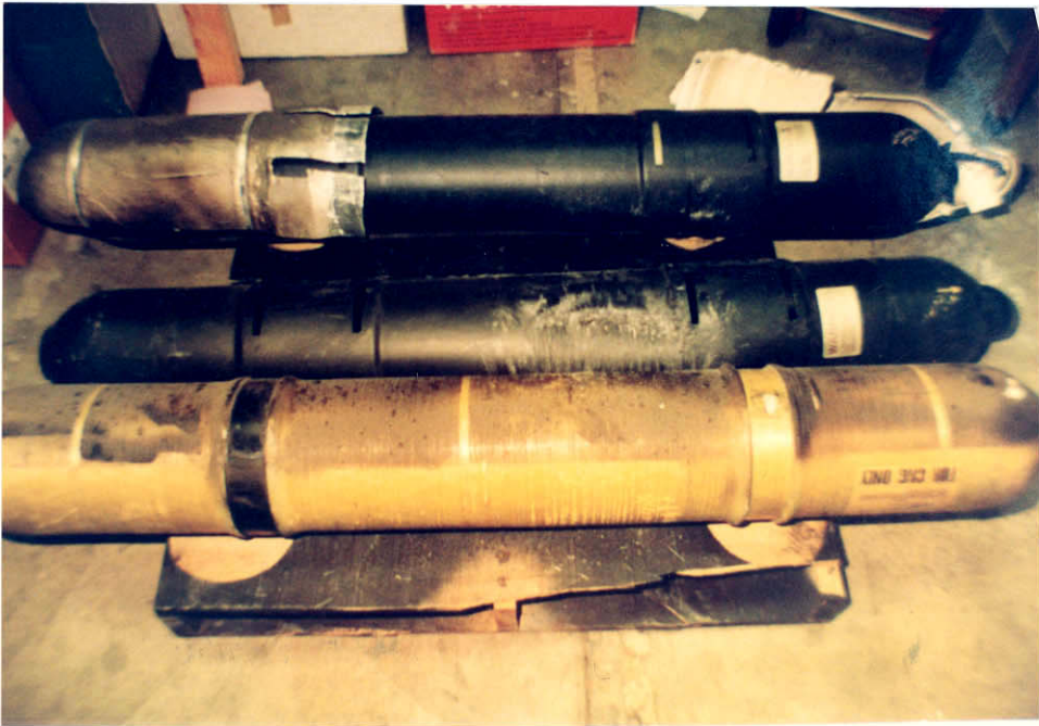
27. Removed Center and Right Cylinders and the Respective HDPE Shields
